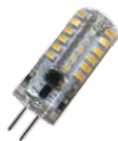
Model: LED-T3-2.0W-30K-ENC Wattage: 2.0W Compare To: 20W Lumens: 225 Size: 3/8" W x 1" L Kelvin: 3000K
